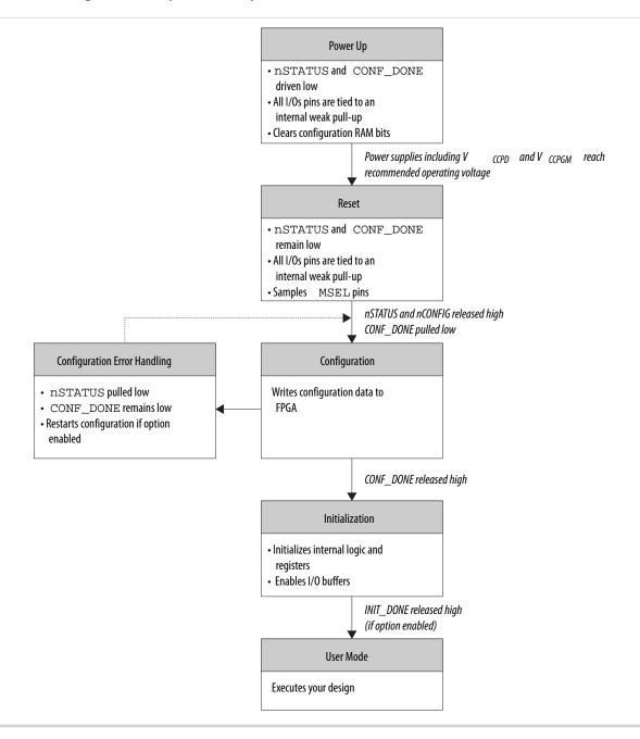
You can initiate reconfiguration by pulling the nconfig pin low to at least the minimum t<sub>CFG</sub> low-pulse width except for configuration using the partial reconfiguration operation. When this pin is pulled low, the nstatus and conf\_done pins are pulled low and all I/O pins are tied to an internal weak pull-up.
