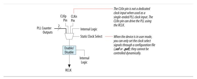
You can set the input clock sources and the clkena signals for the GCLK and RCLK network multiplexers through the Quartus Prime software using the ALTCLKCTRL IP core.
