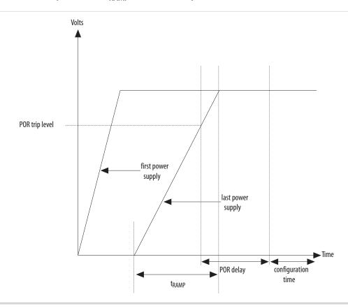
The Cyclone V POR circuitry uses an individual detecting circuitry to monitor each of the configuration-related power supplies independently. The main POR circuitry is gated by the outputs of all the individual detectors. The main POR signal is asserted when the power starts to ramp up. This signal is released after the last ramp-up power reaches the POR trip level during power up.
