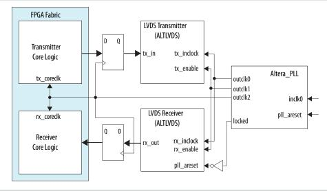
When generating the Altera\_PLL IP core, the **Left/Right PLL** option is configured to set up the PLL in LVDS mode. Instantiation of pll\_areset is optional.
