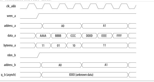
In the dual-port RAM mode, the mixed-port read-during-write operation is supported if the input registers have the same clock. The output value during the operation is "unknown."
