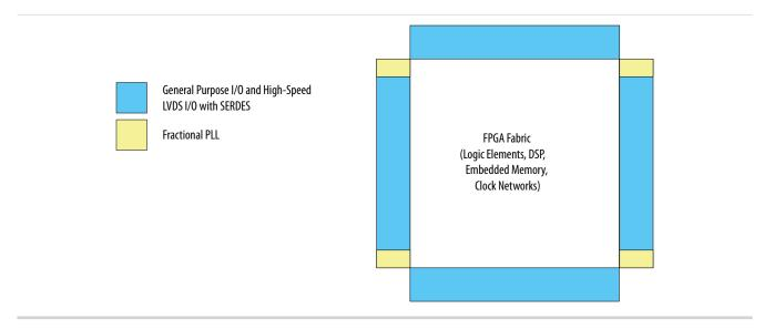
Figure 5-30: High-Speed Differential I/O Locations in Cyclone V GX C3 Devices
