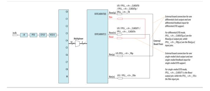
Figure 4-32: Example of Phase Relationship Between the PLL Clocks in EFB Mode
