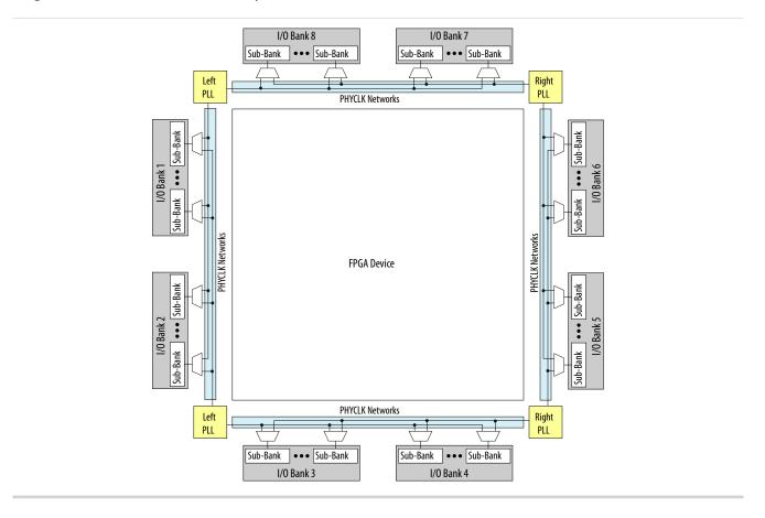
Figure 6-9: PHYCLK Networks in Cyclone V GX C3 Devices
