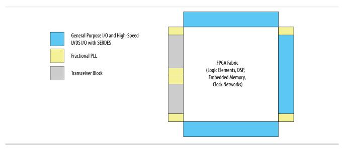
Figure 5-32: High-Speed Differential I/O Locations in Cyclone V SE A2, A4, A5, and A6 Devices
