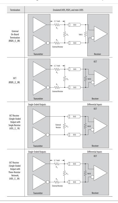
To meet the RSDS or mini-LVDS specifications, you require a resistor network to attenuate the output-voltage swing.
