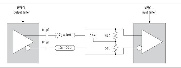
Support for DC-coupled LVPECL is available if the LVPECL output common mode voltage is within the Cyclone V LVPECL input buffer specification.
