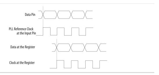
The source synchronous mode compensates for the delay of the clock network used and any difference in the delay between the following two paths:
