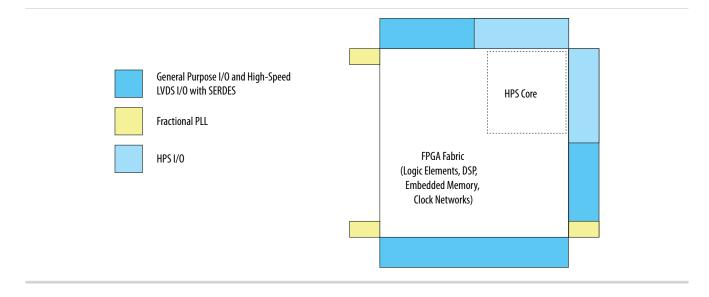
Figure 5-33: High-Speed Differential I/O Locations in Cyclone V SX C2, C4, C5, and C6 Devices, and Cyclone V ST D5 and D6 Devices
