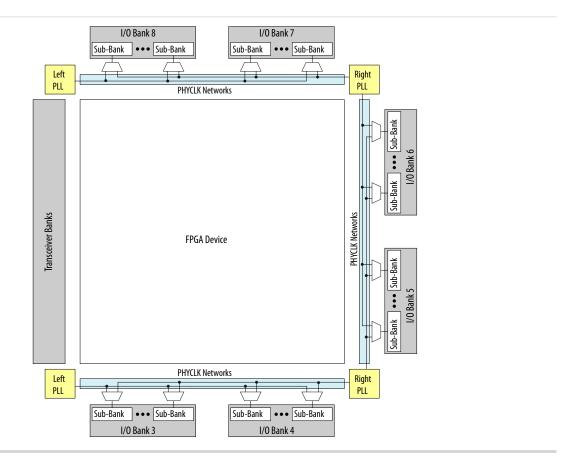
Figure 6-11: PHYCLK Networks in Cyclone V SE A2, A4, A5, and A6 Devices
