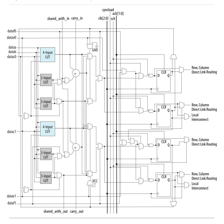
Logic Array Blocks and Adaptive Logic Modules in Cyclone V Devices
