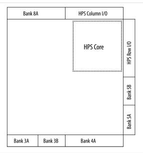
Figure 5-9: I/O Banks for Cyclone V SX and ST Devices
