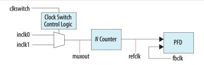
You can delay the clock switchover action by specifying the switchover delay in the ALTERA\_PLL IP core. When you specify the switchover delay, the clkswitch signal must be held high for at least three inclk cycles plus the number of the delay cycles that has been specified to initiate a clock switchover.
