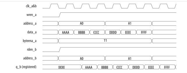
Figure 2-4: Mixed-Port Read-During-Write: Old Data Mode
