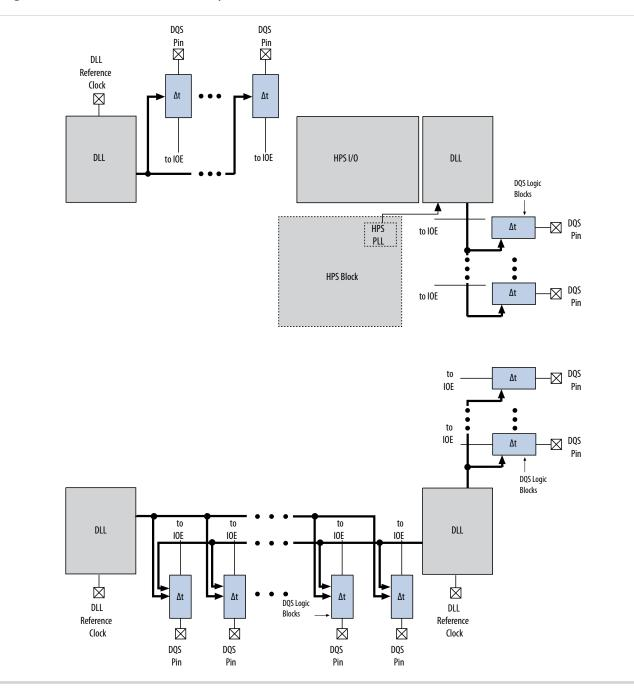
Figure 6-6: DQS Pins and DLLs in Cyclone V SX (C2, C4, C5, and C6) and ST (D5 and D6) Devices
