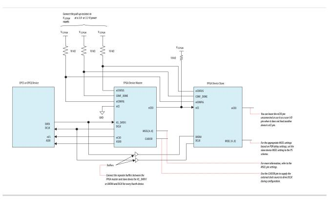
When a device completes configuration, its nCEO pin is released low to activate the nCE pin of the next device in the chain. Configuration automatically begins for the second device in one clock cycle.
