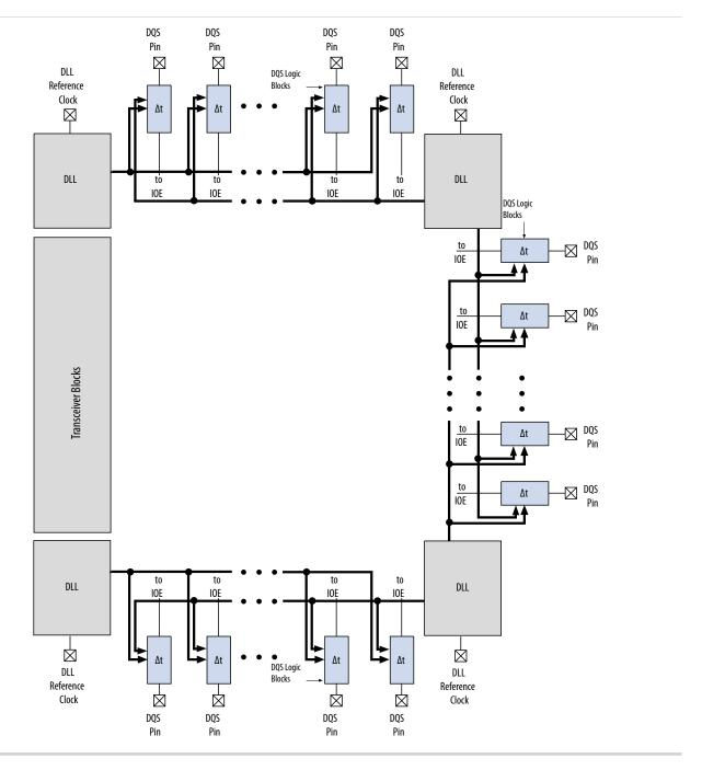
Figure 6-5: DQS Pins and DLLs in Cyclone V SE (A2, A4, A5, and A6) Devices
