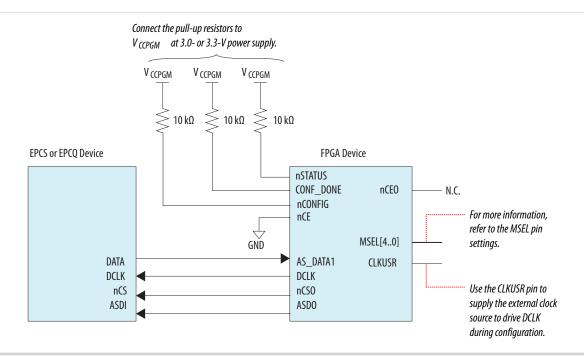
Figure 7-10: Single Device AS x4 Mode Configuration
