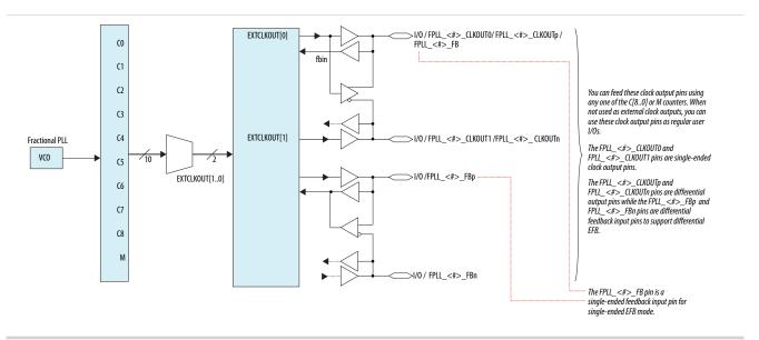
Each pin of a single-ended output pair can be either in-phase or 180° out-of-phase. To implement the 180° out-of-phase pin in a pin pair, the Quartus Prime software places a NOT gate in the design into the IOE.
