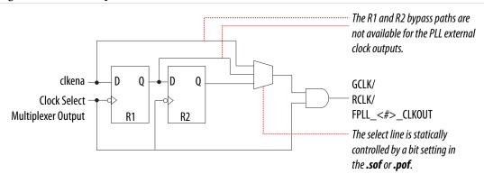
The clkena signals are supported at the clock network level instead of at the PLL output counter level. This allows you to gate off the clock even when you are not using a PLL. You can also use the clkena signals to control the dedicated external clocks from the PLLs.
