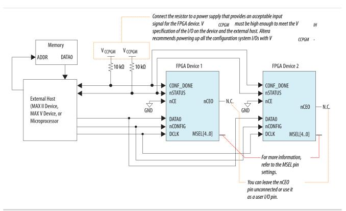
The nCE pins of the devices in the chain are connected to GND, allowing configuration for these devices to begin and end at the same time.
