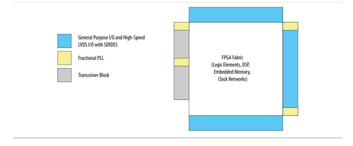
Figure 5-31: High-Speed Differential I/O Locations in Cyclone V GX C4, C5, C7, and C9 Devices, and Cyclone V GT D5, D7, and D9 Devices
