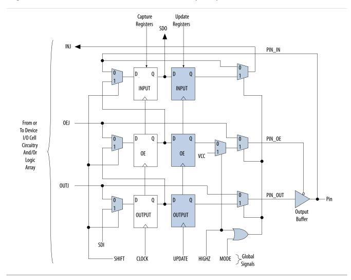
Note: TDI, TDO, TMS, and TCK pins, all VCC and GND pin types, and VREF pins do not have BSCs.
