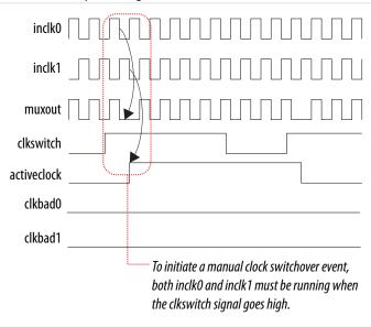
In automatic override with manual switchover mode, the activeclock signal mirrors the clkswitch signal. Since both clocks are still functional during the manual switch, neither clkbad signal goes high. Because the switchover circuit is positive-edge sensitive, the falling edge of the clkswitch signal does not cause the circuit to switch back from inclk1 to inclk0. When the clkswitch signal goes high again, the process repeats.
