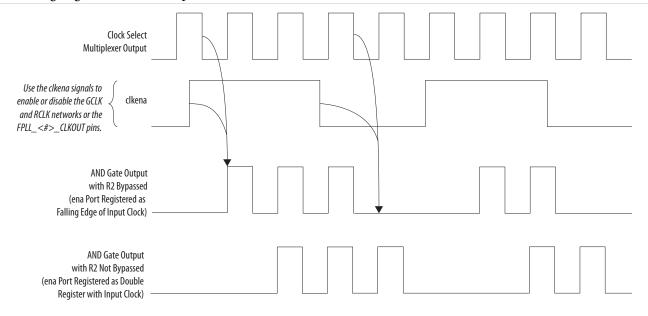
Cyclone V devices have an additional metastability register that aids in asynchronous enable and disable of the GCLK and RCLK networks. You can optionally bypass this register in the Quartus Prime software.
