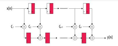
Cyclone V variable precision DSP blocks support the following systolic FIR structures:
