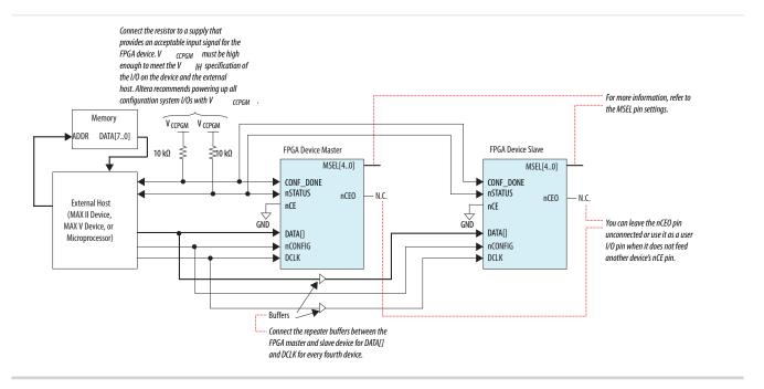
The nCE pins of the device in the chain are connected to GND, allowing configuration for these devices to begin and end at the same time.
