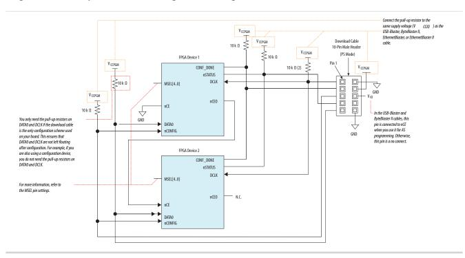
When a device completes configuration, its nCEO pin is released low to activate the nCE pin of the next device. Configuration automatically begins for the second device.
