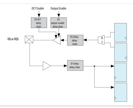
Each DQS logic block contains a delay chain after the dqsbusout output and another delay chain before the dqsenable input.
